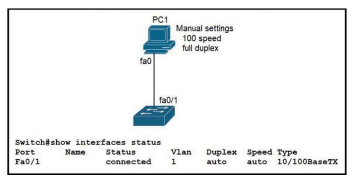
The link between PC1 and the switch is up, but it is performing poorly. Which interface condition is causing the performance problem?
